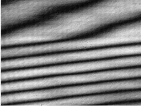
Fig. 2. Fringe pattern of the c-d interface at 0.856 K.
